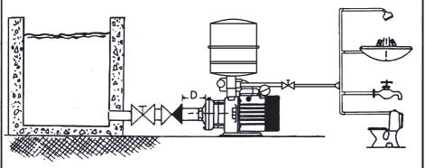
• Check valve at Suction side must be with a minimum distance of 4 x diameter of inlet pipe from the suction port
