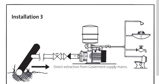
• Direct extraction from Government supply mains usually against regulation, therefore we recommend installation of suction tank as per installation 2
